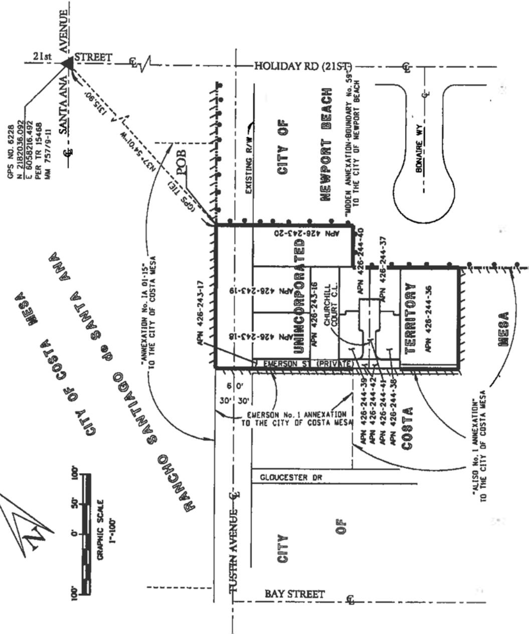
UNLESS OTHERWISE NOTED, ALL DISTANCES ON THIS MAP ARE GROUND AND ARE BASED UPON THE CALIFORNIA COORDINATE SYSTEM (CCS83), ZONE VI, 1983 NAD 1893.35 EPOCH DGS GPS ADJUSTMENT. TO OBTAIN GRID DISTANCE, MULTIPLY GROUND DISTANCE BY 0.999869372
