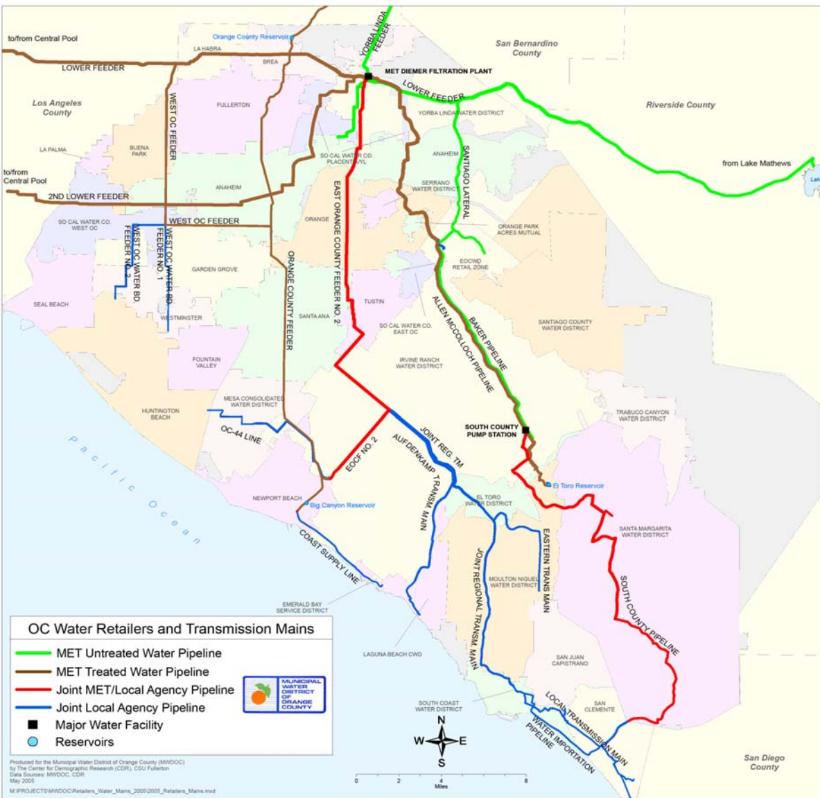
Figure 5.1, Orange County Water System
